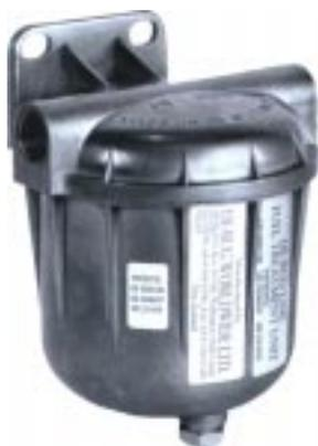
There are three vertically stacked ceramic magnets inside the DeBug L500 unit. As fuel passes through the many pathways between these magnets, microbes in the fuel are exploded by 24 rapid magnetic field changes. Their remains pass harmlessly through the fuel filter and are burnt by the engine.
